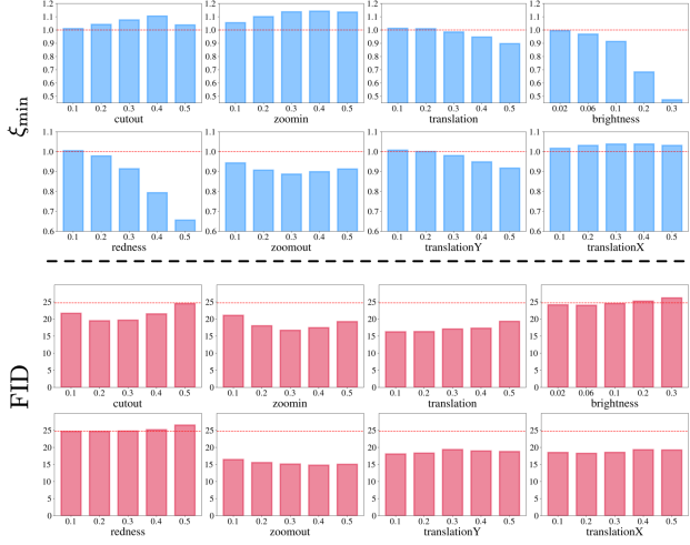
Figure 4. (Top) The values of \xi_{\min} for augmented versions of CIFAR-10 for different values of the augmentation strength. We normalize them dividing by \xi_{\min} \approx 0.0042 of the non-augmented version of the dataset. (Bottom) The FID values of a SNDCGAN (BCR) trained on the corresponding dataset. The values are taken from Zhao et al. (2020). For \xi_{\min} a higher value is “better” in terms of connectivity of dataset and theoretical convergence. For FID smaller values are better. In most cases we observe a negative rank correlation between \xi_{\min} and FID.
